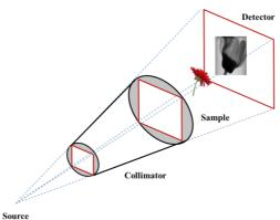
Figure 1: Schematic of Neutron Imaging set-up
