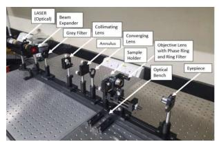
Figure 1: Experimental set up for PCM
