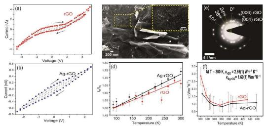
**Fig.1** I-V curves obtained upon illumination with 532 nm for (a) rGO and (b) Ag-rGO. (c) FESEM micrograph of Ag-rGO nanocomposite. (d) Variation of ID/IG ratio with temperature for rGO and Ag-rGO. (e) SAED pattern where angle between the spots corresponding to rGO plane is shown. (f) Variation of κ with temperature for rGO and Ag-rGO.
