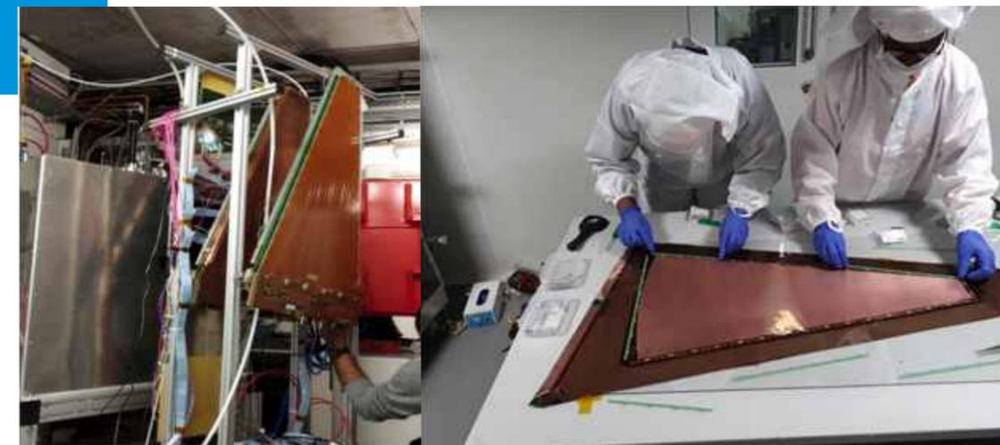
Fig. 4: (left) Two GEM chambers are ready to take data at GSI-Germany (right) a GEM chamber being assembled at VECC-Kolkata
