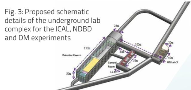
Fig. 3: Proposed schematic details of the underground lab complex for the ICAL, NDBD and DM experiments
