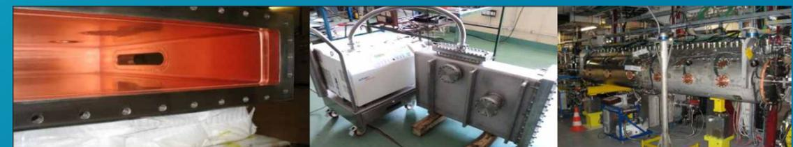
7)Copper coated SS Power Couplers developed at RRCAT & Installed in Linac 4 at CERN
