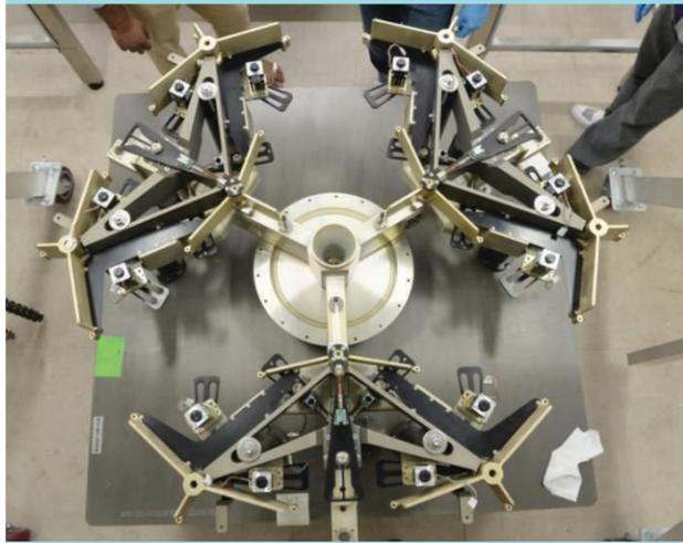
Figure3: **Prototype SSA** fabricated in India (Credits: IIA/ITCC/ Fred
