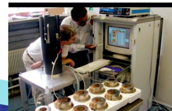
Superconducting corrector magnets for LHC
