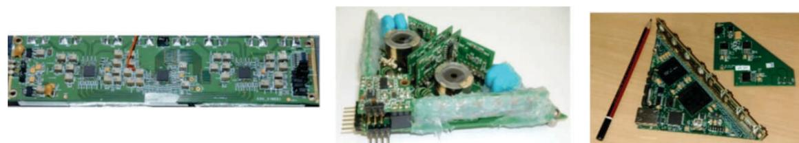
Fig. 12: (L to R) Front-end electronics board with 8-channel amplifier and discriminator, ±5kV DC module, DAQ board. All developed in house.
