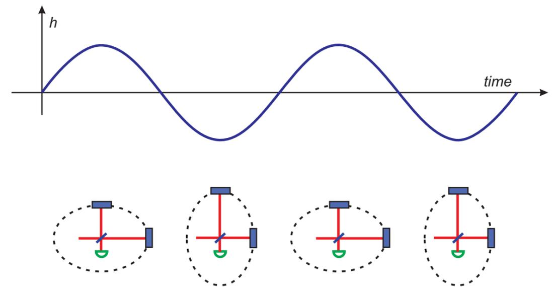
Effect of a passing gravitational wave on the L shaped arms of an interferometer
