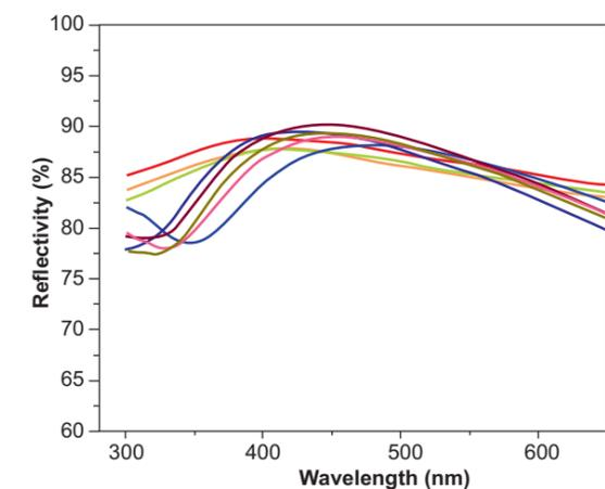
Fig.2 Plot of reflectivity as a function of wavelength for a test sample of 8 mirror facets.
