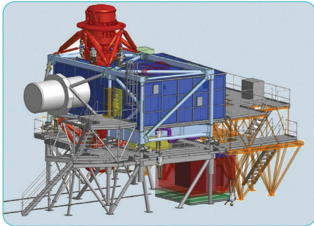
Figure 9: Internal design of NFIRAOS. The three potential instrument output ports are seen.
