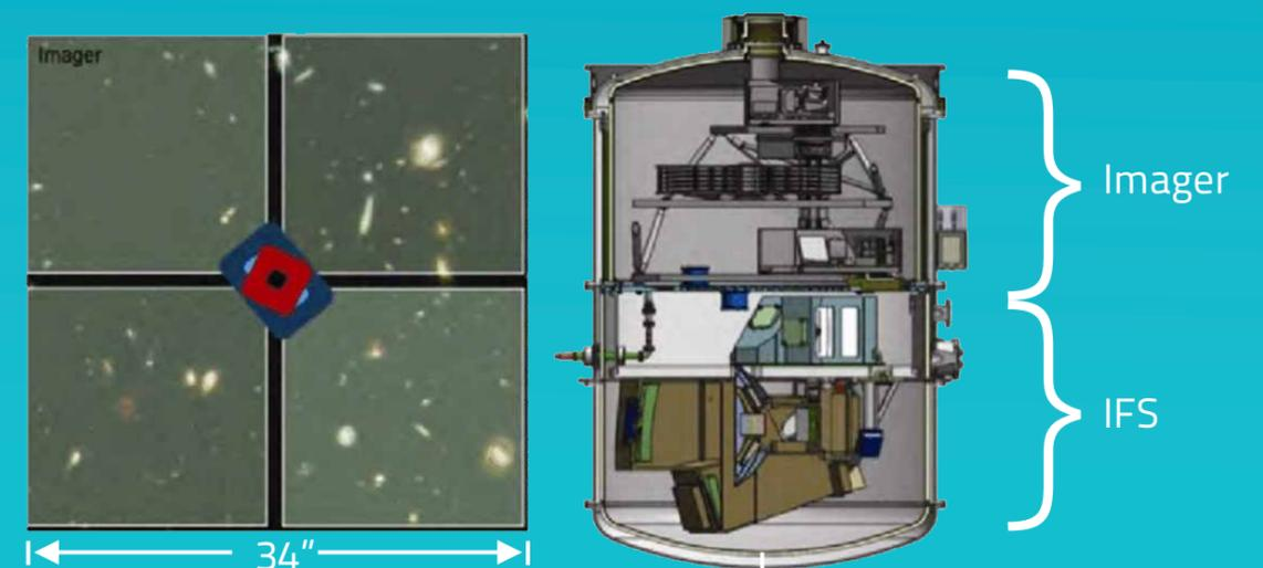
Figure 8: (Left) The IRIS field of view. Four 4k x 4k detectors are used for the diffraction-limited imager. The coloured rectangles in the centre represent the four options for the field of view of the integral field spectrograph (IFS). (Right) The two-part design of the science instrument with light entering from above. The imager and IFS are being built separately and will be integrated before the instrument is sent to the telescope site.
