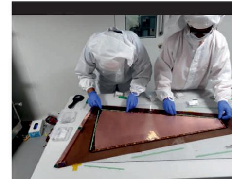
GEM prototype fabrication at VECC
