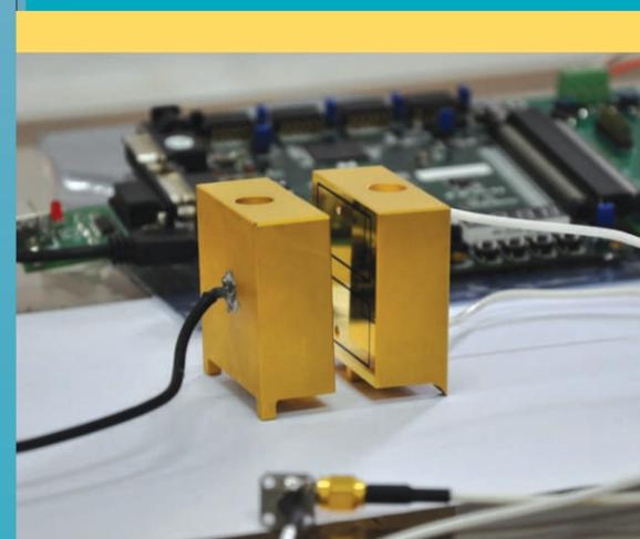
Figure2: **Prototype Edge Sensor** fabricated in India. (Photo credits: IIA/ITCC/ Prasanna Deshmukh).
