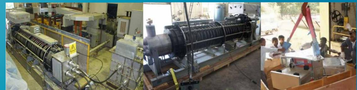
5)1MW klystron test stand at RRCAT
