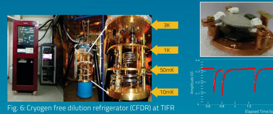
Fig. 6: Cryogen free dilution refrigerator (CFDR) at TIFR
