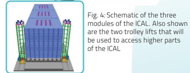
Fig. 4: Schematic of the three modules of the ICAL. Also shown are the two trolley lifts that will be used to access higher parts of the ICAL
