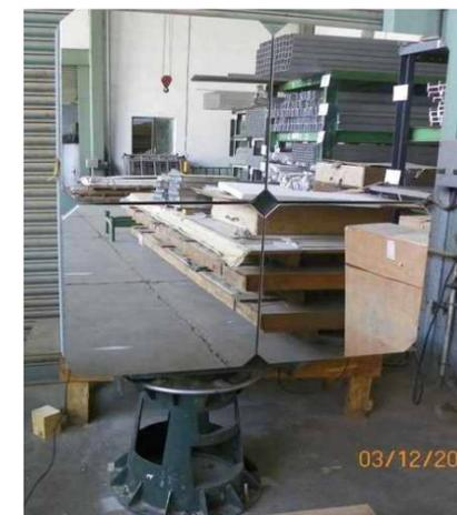
Fig.1 Photograph of one mirror panel comprising 4 aligned spherical mirror facets.
