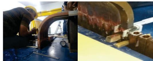
Fig. 10: Induction brazing of the upper C-section to the U-Sections of 30mm x 30mm OFHC copper conductor of 17mm bore through which cooling water will be pumped.
