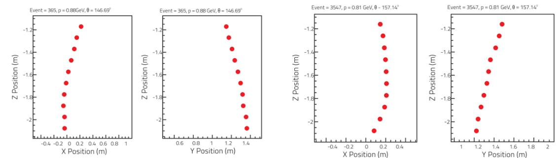
Fig. 14: Examples of cosmic muons, of either charge, firing various layers of the RPC's (at various Z positions) caused by their traversing the mini-ICAL detectors from top to bottom. The bending can be seen in the X-positions but essentially no bending in the Y-positions.
