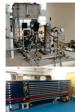
Fig 13: Low conductivity chilled water system for cooling the current carrying coils of the mini-ICAL magnet (left) and a view of the assembled mini-ICAL (right)
