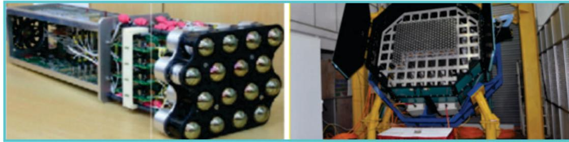
Fig.3 A fully assembled 16 channel Camera integrated module of MACE telescope.
