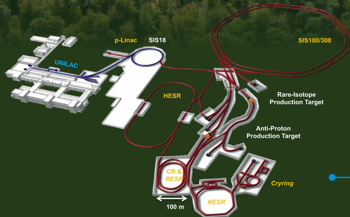
Fig.1: Schematic view of the FAIR facility. GSI is shown at the left. Beams from GSI will be injected to the main SIS100 ring and after acceleration will cater to four physics pillars. The switching building after SIS100 is crucial in delivering beams to different research facilities in parallel.
