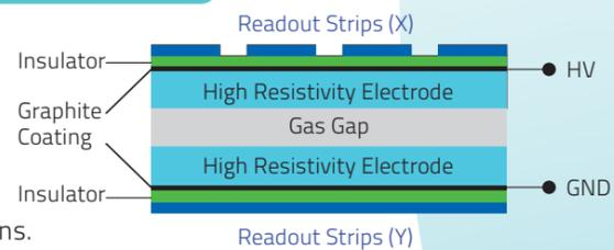
Fig. 5: Schematic of a Resistive Plate Chamber (RPC) that will detect charged particles such as muons.
