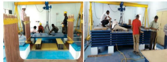
Fig 9: mini-ICAL coil and magnet assembly in progress, using a gantry crane
