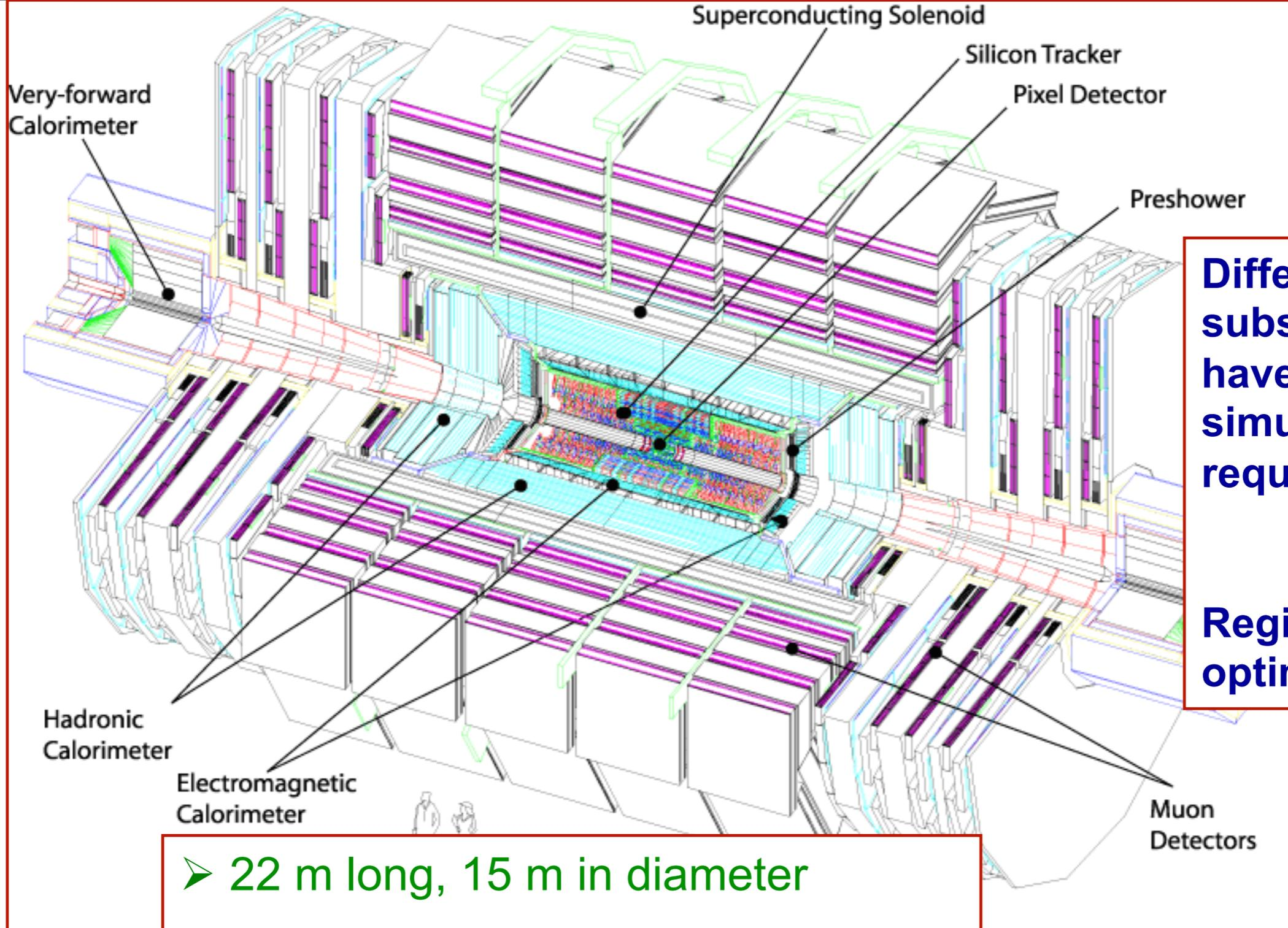
**Different subsystems have different simulation requirements**
