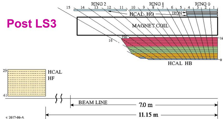
Layer grouping of HB/HE has changed with time (depending on readout scheme)
