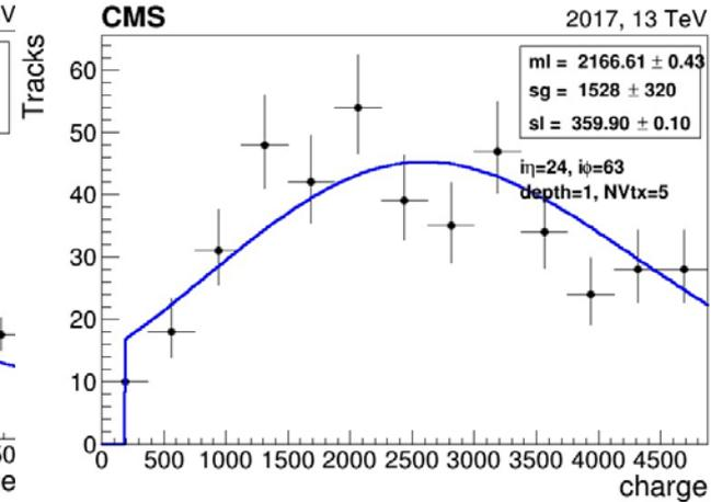
Charge distribution due to muon in  $i\eta=24$  depth=1 in different bins of  $N_{vtx}$
