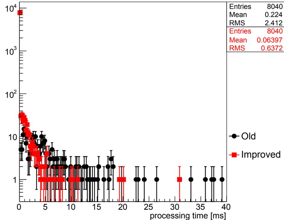
There is a tail in the timing plot (more for HE). This tail is investigated and is due to large number of PixelTracks. These events do not eventually provide any good isolated tracks at the offline stage. A simple filter can be made to remove this tail
