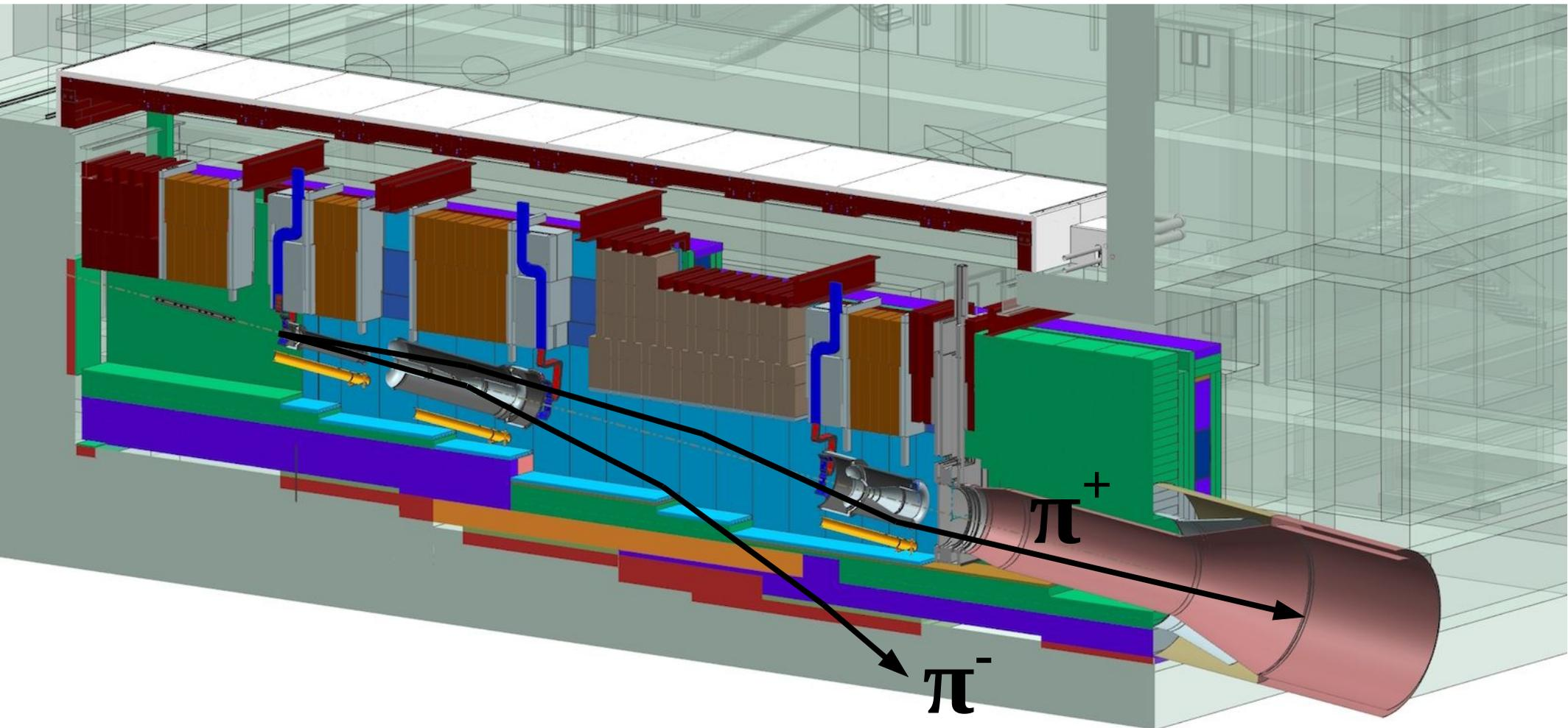
Magnetic horns focus one sign into a decay pipe, and defocus the other
